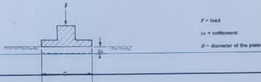
The diameter  $D$  of the plate is generally 0.30 m. For very coarse grained material also plates with diameter  $D = 0.60$  m and  $D = 0.762$  m are used
