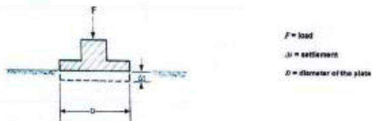
The diameter  $D$  of the plate is generally 0.30 m. For very coarse grained material also plates with diameter  $D = 0.60$  m and  $D = 0.762$  m are used.
