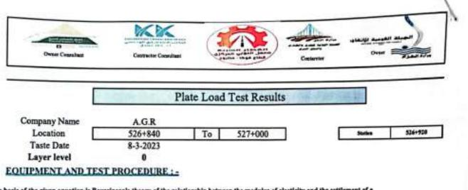
The load is applied to a circular rigid steel bearing plate by a hydraulic jack in several steps. The settlement under each load step is recorded. The following sketch shows the principle of the test.
