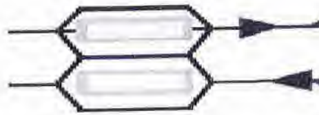
Figure 1: 660 meter long usable length for freight loops
